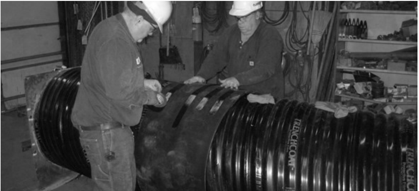
Over lap strip flat gaskets and use duct tape to join.
