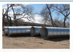
Aluminized Type 2 (ALT2) CMP has been rigorously studied and installed for over 60 years across a wide range of environments. Backed by state DOTs, national agencies, and field data, ALT2 offers a minimum of 2x (up to 8x) the service life of galvanized steel, providing 75+ years of performance within the recommended environmental ranges (5-9 pH range and  $\ge 1500$  ohm $\bullet$ cm site conditions).
