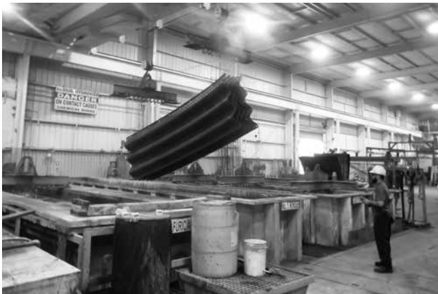
Black Steel MULTI-PLATE before the Zinc Tank
