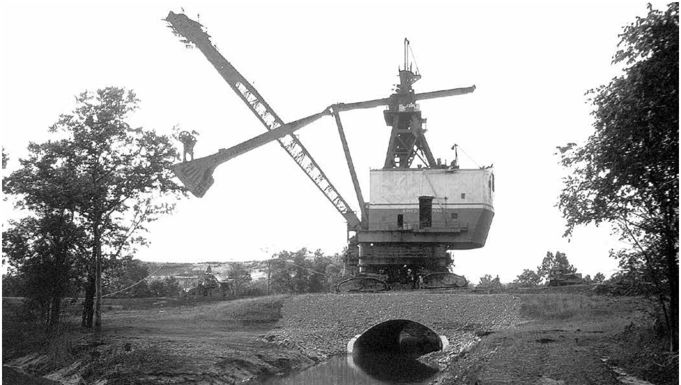
"The Chief" a 5,000,000 lb. drag line over steel SUPER-SPAN™ at Peabody Coal in Zanesville, Ohio
