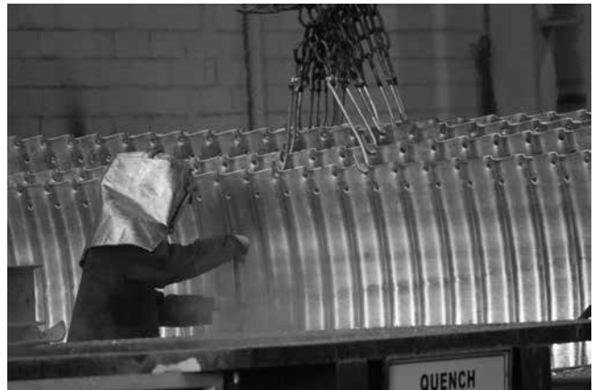
Galvanized MULTI-PLATE removed from the Zinc Tank
