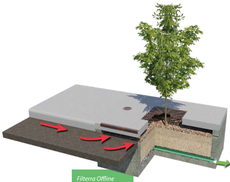
Filterra Offline Bypass via downstream catch basin.
